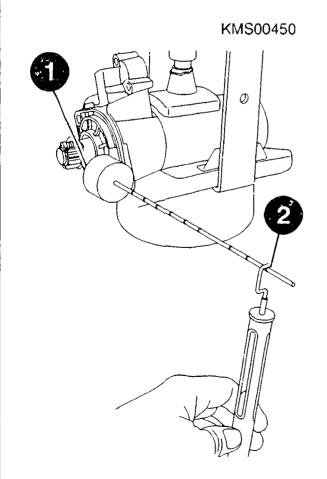
Checking clutch overrunning torque
